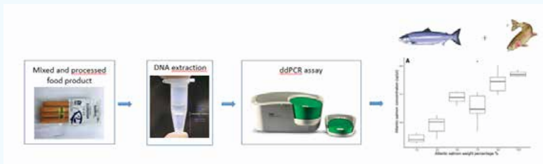
Figure 2 Identification of mixed salmon samples via ddPCR. A sample that can contain several salmon species is used to perform DNA extraction, then the DNA is added to a ddPCR mix in which primers and a probe are added that only multiply a piece of mitochondrial DNA from Atlantic salmon ( Salmo salar ). In test samples in which tissue from S. salar and Oncorhynchus mykiss were mixed in different proportions, the number of copies of DNA from the ddPCR was found to be correlated with the weight percentage of Salmo salar tissue added to the mixture.
