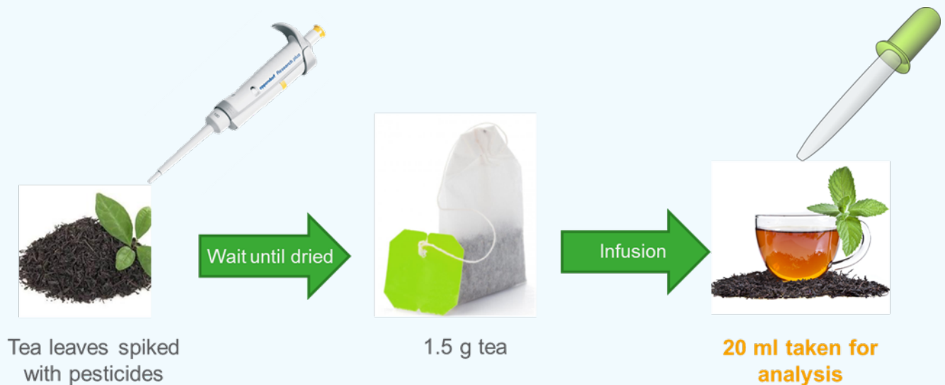
Figure 1. Preparation protocol for the analysis of pesticides in tea brew
