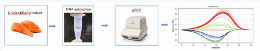
Figure 1 Identification of salmon samples via HRMA and qPCR. A piece of salmon fillet from one species is used to perform DNA extraction, then the DNA is added to a qPCR mix where primers are added so that only a piece of mitochondrial DNA from salmon species is multiplied. The DNA sequence of this piece is different for each salmon species, resulting in a specific melting curve.
